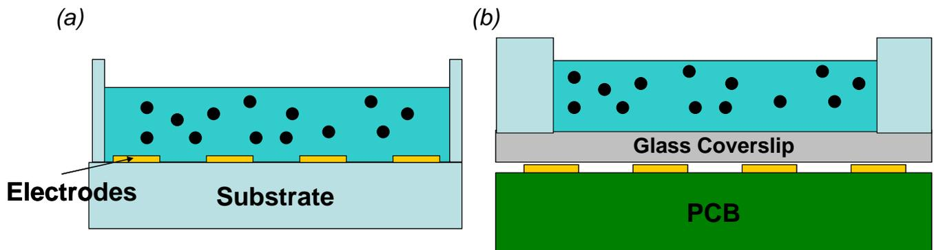
**Fig. 2.** (a) A schematic diagram of the conventional approach in implementing DEP. Electrodes and substrate should be disposed of after each experiment. (b) A schematic diagram of the PCB-based DEP implementation. DEP electrodes are easily fabricated on a PCB and can be reused again and again since the electrodes are not in direct contact with the sample.
