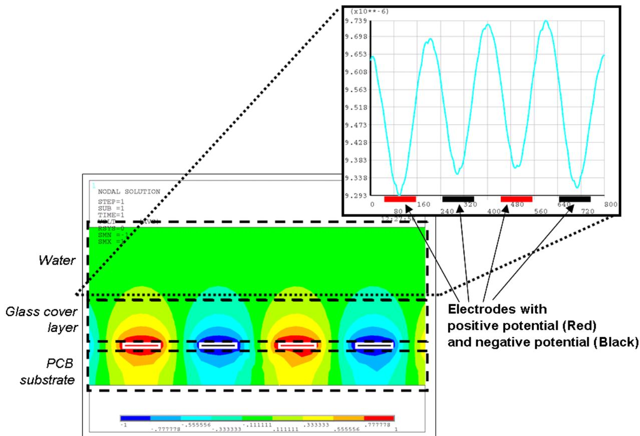
**Fig. 3:** Numerical analysis of the electric potential generated by the PCB electrodes. Electrodes in red and in black are set to +1V and -1V respectively. *Inset:* Square of the electric field magnitude,  $|E|^2$ , on the dotted line 10 $\mu$ m above the glass cover layer. Black and red bar shows the position of the electrodes. The electric field intensity is weakest at the center of the electrode and strongest between the electrodes.
