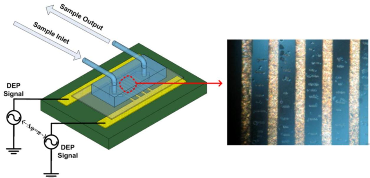
**Fig. 4:** The device is made from a PCB and a thin glass coverslip. The glass coverslip serves as an insulator between the solution and the electrode pattern.
