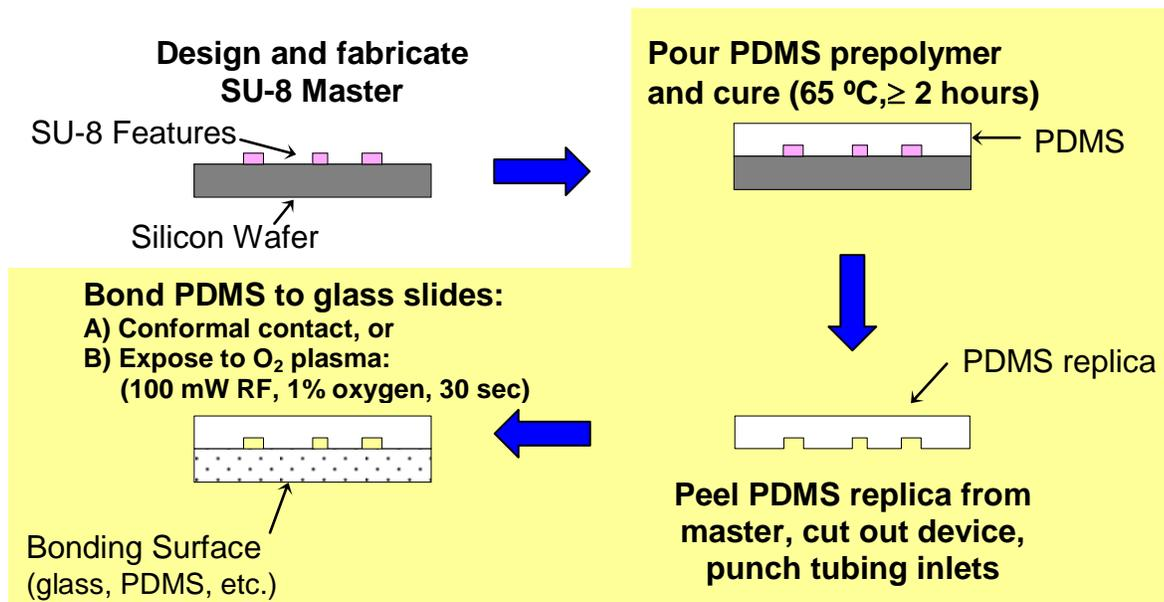
**Scheme 1.** Schematic overview of PDMS Device Fabrication.
