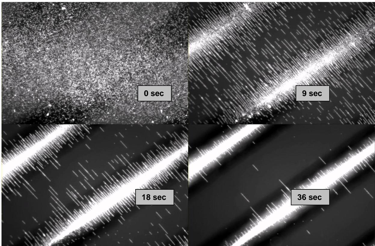
**Fig. 5.** Dark field images of the fluorescently labeled 3µm polystyrene beads during DEP. The trajectories of the polystyrene beads are visible as short lines, indicating the traveled distance during exposure time of the camera. After applying the AC voltages for 36 seconds, most of the beads become focused on top of the electrodes by negative DEP force
